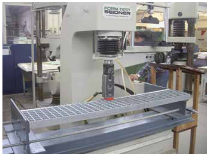
Fig. 31: Test arrangement prior to the application of a load
